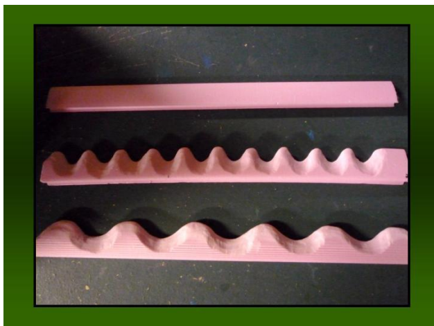
Left: Three different blade edges tested; Right: The edges mounted on tested wind blades.
